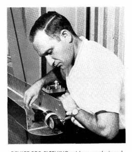
DEVICE FOR SLEEVING cables was designed at Livermore,
